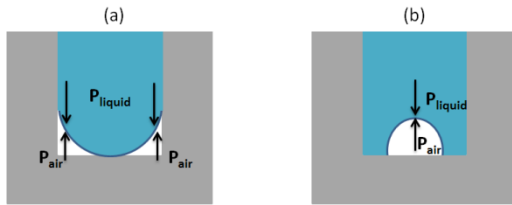
Figure 11 – Pressure equilibrium between trapped air ( P_{\text{air}} ) pockets and suspended liquid ( P_{\text{liquid}} ) inside the DTI for (a) hydrophobic surface and (b) hydrophilic surface
