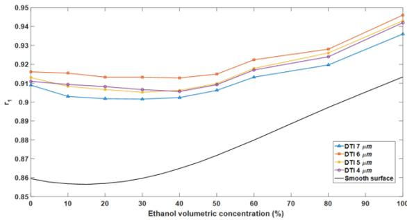
Figure 7 – Variations of the acoustic reflection coefficient  $r_l$  on the bottom of the DTI 4, 5, 6 and 7  $\mu\text{m}$  for different distilled water / ethanol mixtures injected inside the 80  $\mu\text{m}$  micro-channel.
