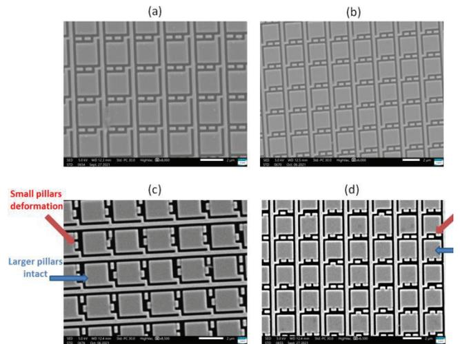
Figure 13 – SEM images of the DTI matrix showing the etched trenches (black color) and the silicon pillars (grey color) for (a) 4  $\mu\text{m}$ , (b) 5  $\mu\text{m}$ , (c) 6  $\mu\text{m}$  and (d) 7  $\mu\text{m}$  etch depth
