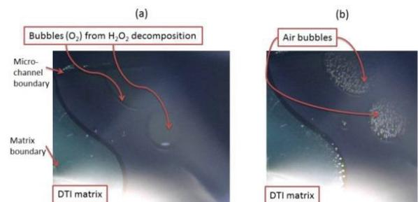
Figure 9 – (a) Observed bubbles during the injection of the SC1 solution in the micro-channel (b) air bubbles exiting the DTI network during the drying phase.
