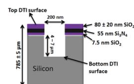
Figure 2 – Schematic of the trench structure
