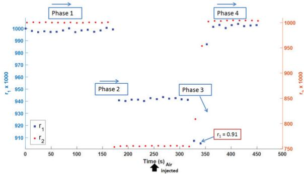
Figure 10 – Variation of the acoustic reflection coefficients  $r_1$  and  $r_2$  with time for DTI 4  $\mu\text{m}$  with 80  $\mu$  micro-channel injected with pure ethanol: initial phase (phase 1), injection of liquid (phase 2), wetting transition to complete wetting (phase 3) and complete drying (phase 4)
