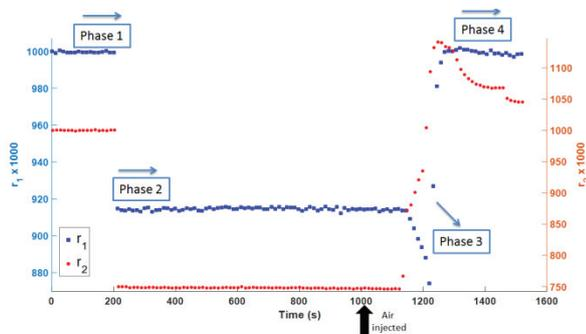
Figure 8 – Variation of the acoustic reflection coefficients  $r_1$  and  $r_2$  with time for DTI 6  $\mu\text{m}$  with 80  $\mu\text{m}$  micro-channel injected with SC1 solution: initial phase (phase 1), injection of liquid (phase 2), wetting transition (phase 3) and complete drying (phase 4)
