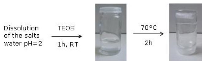
Fig. 1 Hydrolysis of TEOS in the presence of the salts and sol-gel transition. Sol in the middle, gel on the right.
