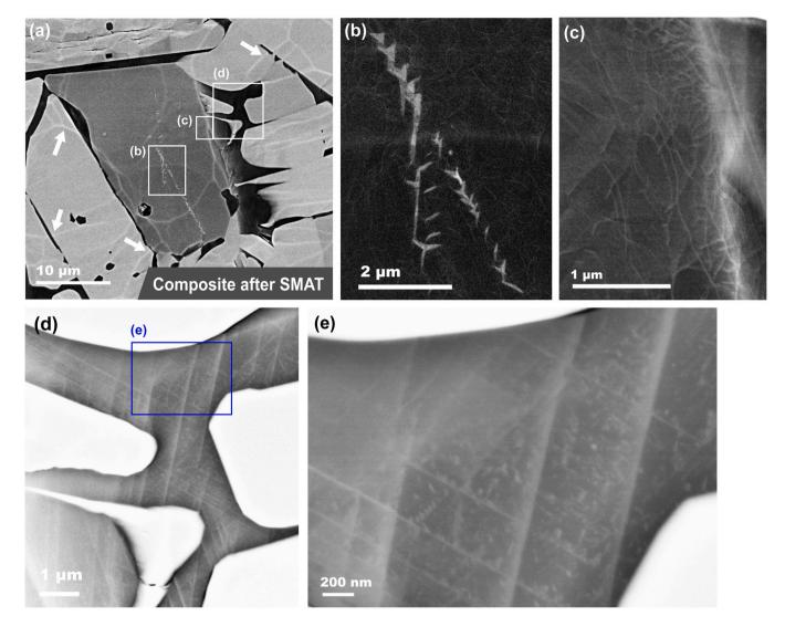
Fig. 6. BSE micrographs of the composite material in ECCI conditions. (b) dislocation wall within Ti<sub>3</sub>AlC<sub>2</sub> (c) and dislocation networks near the grain boundary. (d,e) Parallel straight-lined defects in TiAl<sub>2</sub>.
