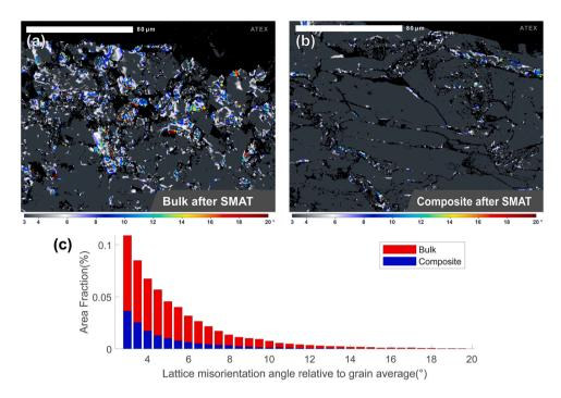
**Fig. 5.** Lattice misorientation relative to grain average orientation, drawn in ATEX software from EBSD maps. (a) shows the deformed *bulk*, (b) shows the deformed *composite*. (c) plots a wider area fraction of misorientations within the *bulk*.
