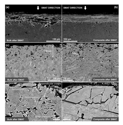
Fig. 3. BSE micrographs of bulk material (a,c,e) and composite material (b,d,f.) after SMAT. (a,b) surface aspect; (c,d) cross section of the surface and subsurface showing the affected zone; (e,f) higher magnification images showing structural defects at the treated surface.
