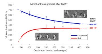
**Fig. 4.** Vickers microhardness gradients measured from the surfaces treated by SMAT. The insets show SEM micrographs of indentations left in the *composite* and *bulk* materials.
