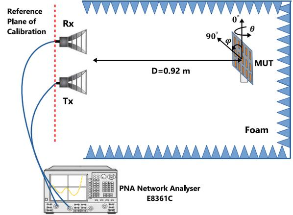
Figure 10: Free-space measurement setup
