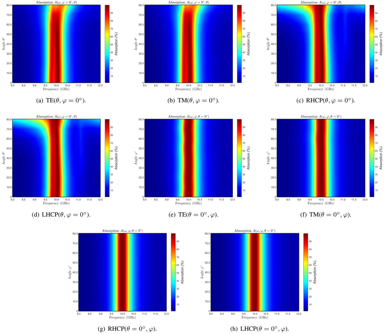
Figure 6: Absorption Spectra of the unit-cell for different polarizations : Elevation angle  $\theta$  test : (a)-Mode TE,(b)-Mode TM,(c)-RHCP and (d)-LHCP. Azimuthal angle  $\varphi$  test (e)-Mode TE, (f)-Mode TM, (g)-RHCP and (h)-LHCP.
