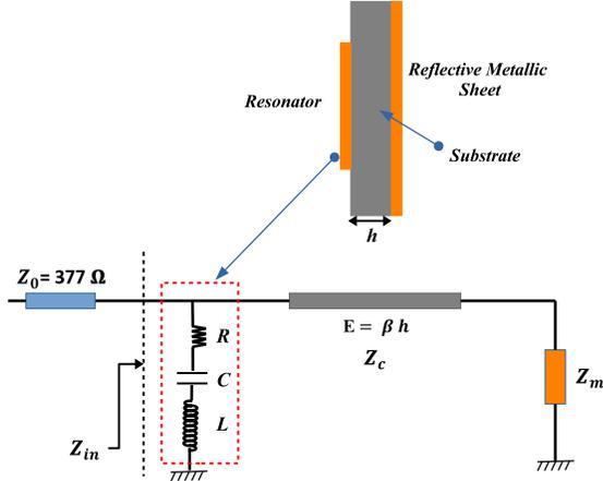
Figure 4: Equivalent circuit model of the unit-cell
