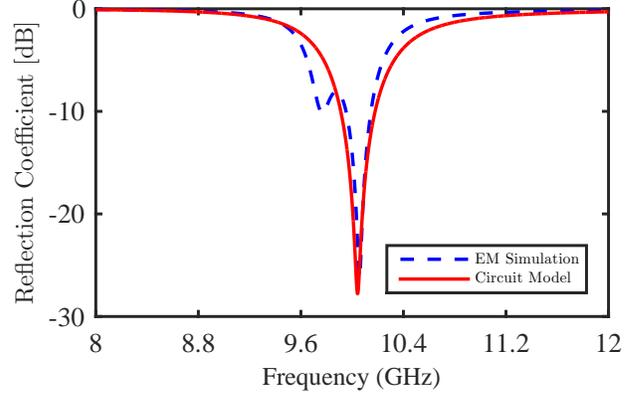
Figure 5: Unit-Cell reflection coefficient : EM Simulation versus circuit model responses
