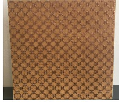
Figure 9: Fabricated metasurface array (12 × 12) cells
