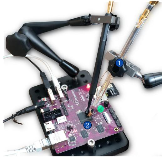
**Figure 5: ULTRA framework is installed with a handcrafted EM-compatible probe ① placed 10mm above Ci20’s processor ② to detect *beurk* rootkit.**
