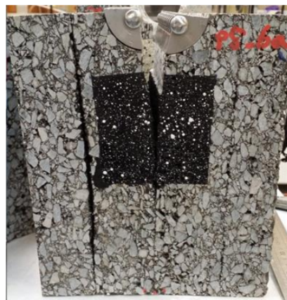
FIG. 2 – Example of secondary debonding during WST of extracted specimens coming from pavement test tract (from [5])
