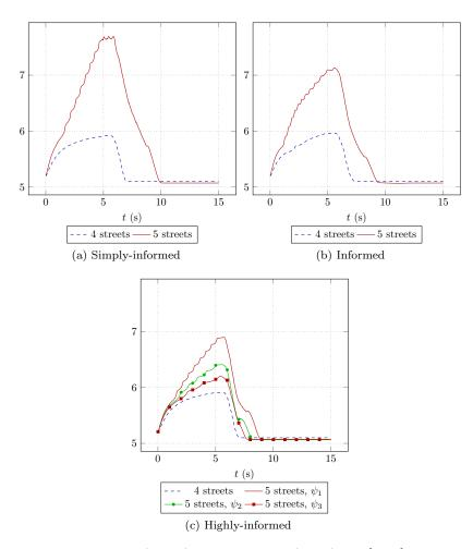
Fig. 7: Braess' network (Fig. 6): travel time  $TT(1, 6, t), t \in [0, 15]$  for different level of information. Here, the parameter  $\epsilon$  of the smooth activation function  $\hat{\psi}$  is set with  $\epsilon = \{1, 2, 3\}$  and called, respectively,  $\psi_1, \psi_2, \psi_3$ .
