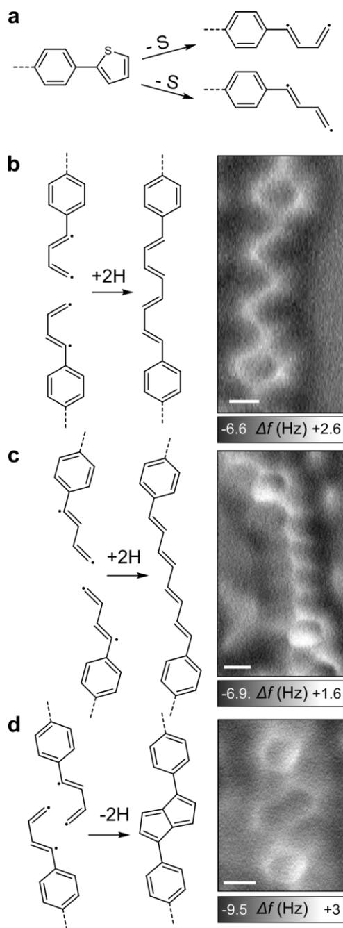
Figure 3. Schematic drawings of the different coupling schemes along with representative high-resolution AFM images. (a) Dissociation of the thiophene rings. Formation of (b) *cis*-oligoacetylene chains, (c) *trans*-oligoacetylene chains and (d) pentalene. Scale bars: 0.2 Å.
