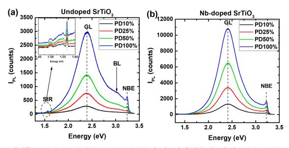
Fig. 7. PL spectra for different excitation intensities (80 K, 325 nm excitation) (a) undoped sample, (b) Nb-doped sample. The excitation intensities are selected by density filters: 100%, 50%, 25%, and 10% transmission. The inset of the panel is a magnified view of SIR spectra.
