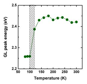
**Fig. 5.** GL peak energy vs. temperature (Nb-doped sample) showing the steep shift at 100–120 K (30 KeV e-beam energy), the transition temperature range is represented by the shaded area.
