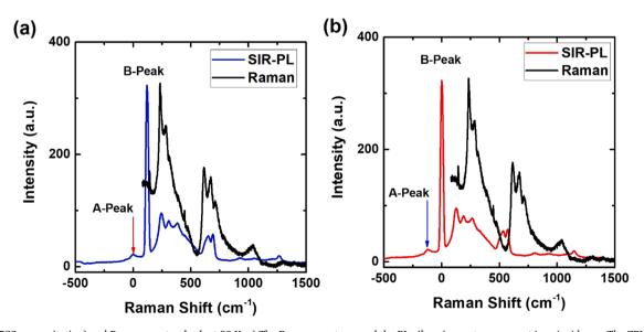
Fig. 12. PL (532 nm excitation) and Raman spectra, both at 80 K. a) The Raman spectrum and the PL vibronic spectrum are put in coincidence. The ZPL fits the peak A of the PL spectrum. b)The B line is taken as the ZPL. In this case, the vibronic PL peaks are fully decoupled from the Raman peaks.
