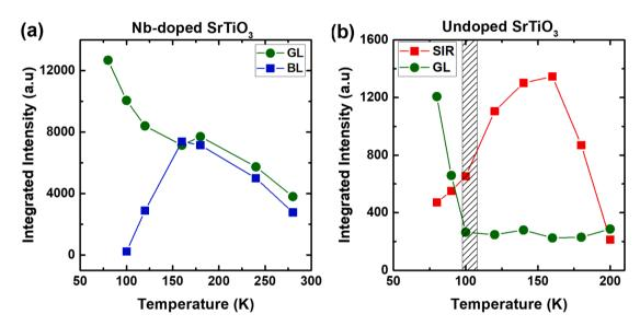
Fig. 4. a) BL and GL CL intensities vs. T (Nb-doped sample), b) GL and SIR CL intensities vs. T (undoped sample) (30 KeV e-beam energy).
