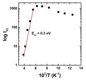
Fig. 14. SIR CL intensity vs. T.
