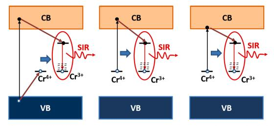
**Fig. 13.** Scheme of the excitation and emission mechanism of the SIR emission. a) intrinsic excitation with either the e-beam (CL) or above bandgap light (325 nm), b) excitation of  $Cr^{3+}$  with subband gap light (532 nm), c) excitation of  $Cr^{3+}$  with subband gap light (633 nm).
