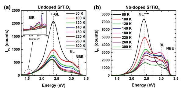
Fig. 8. PL spectra for selected temperatures between 80 and 300 K. a) undoped sample, b) Nb-doped sample. The inset of panel (a) is a magnified view of the SIR spectra.
