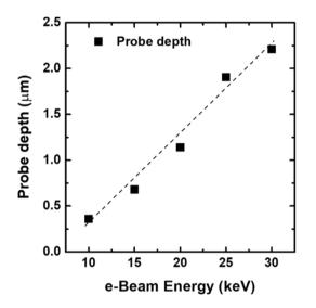
Fig. 2. Maximum electron energy loss (nominal probe depth) calculated by Montecarlo simulation using the Casino software.
