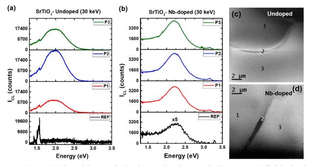
Fig. 11. CL spectra (80 K, 30KeV) in the scratched area. a) undoped sample, spectra taken at the points numbered in Pan-CL image (c), (b) Nb-doped sample, spectra taken at the points numbered in Pan-CL image (d). The spectra taken far away from the scratches are plotted as reference spectra.
