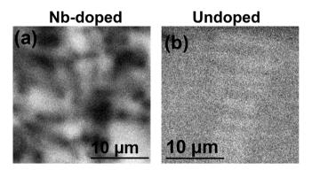
**Fig. 6.** Panchromatic CL (Pan-CL) images of the Nb-doped sample (a) and undoped sample (b). The undoped sample looks homogeneous, while the Nb-doped sample exhibits regions with different contrast; however, the CL spectrum does not show changes between the zones with distinct contrast, other than the intensity.
