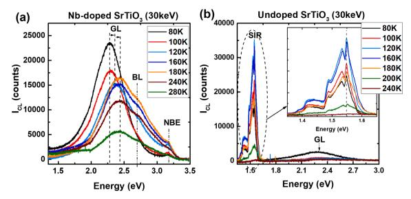
Fig. 3. CL spectra for selected temperatures between 80 and 280 K. a) Nb-doped sample, b) undoped sample (30 KeV e-beam energy).
