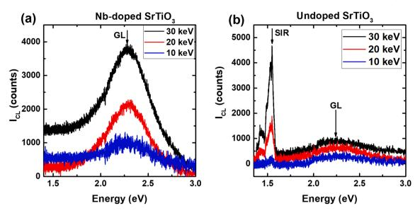
Fig. 1. CL spectra at 80 K for 10, 20 and 30 keV e-beam energies. a) Nb-doped sample, b) undoped sample.
