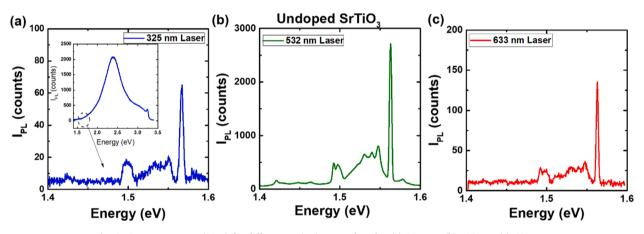
Fig. 9. SIR PL spectrum (80 K) for different excitation wavelengths. (a) 325 nm, (b) 532 nm, (c) 633 nm.
