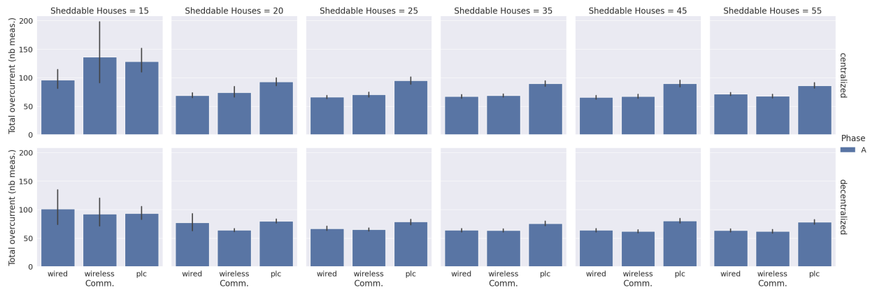
Fig. 4: Total overcurrent versus number of sheddable houses. The current threshold is set to 0.5 kA, message size to 1 kB, shedding duration to 60 s, sampling period to 20 s and latency to 10 ms.
