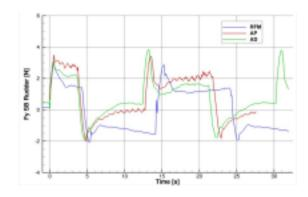
Fig. 9 Time history of transversal force Fy on the starboard rudder (in the frame linked to the rudder)
