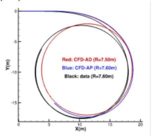
Fig.21 Trajectory of the KCS TC35 motion
