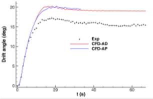
Fig.24 Time history of drift angle for the KCS TC35 motion
