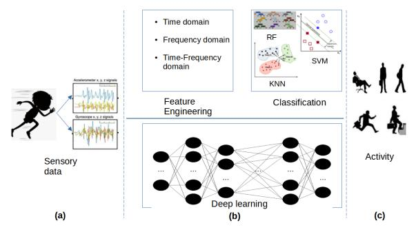
Fig. 1. HAR from IMU sensor data comprises three main parts, (a) data capture and pre-processing (accelerometer and gyroscope data); (b) modeling and training, using either feature engineering with standard classifiers or deep learning extract representations from raw data, and (c) activity recognition.
