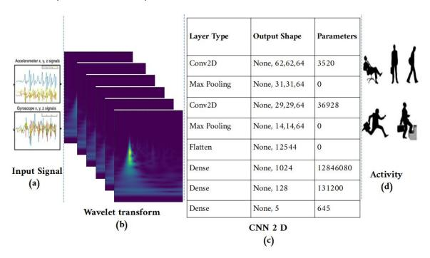
Fig. 2. CWT-CNN2D framework comprises three main parts, (a) data pre-processing for sensor-based HAR (accelerometer and gyroscope); (b) continuous wavelet transform applied on data; (c) training phase, which utilizes CNN2D, and (d) activities recognition.
