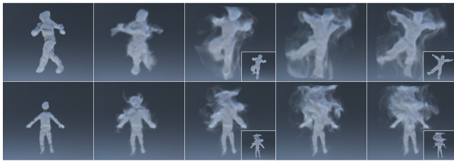
Figure 18: Selected frames of five different smoke simulations where our reconstructed densities are used as keyframes (inset images) to artistically control the motion of the smoke [TACS21]. Due to the underlying fluid solver, intrinsic flow details appear.
