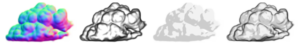
Figure 7: The differentiable sketcher computes normals, contours, and toon shading (from left to right), and combines them into the final sketch (right).
