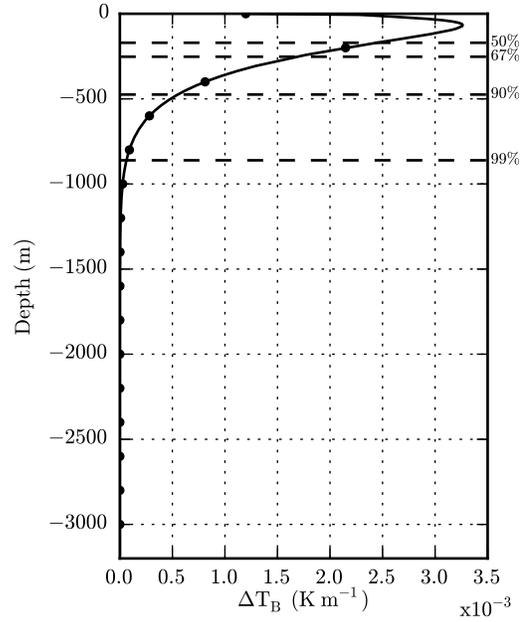
Fig. 7. Contribution of each layer to the total brightness temperature (K m<sup>-1</sup>).
