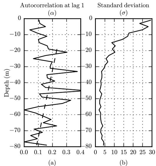
Fig. 4. AR(1) parameters for each 2 m thick layer between the surface and a depth of 80 m: (a) autocorrelation coefficient at lag 1 ( $\alpha$ ) with the regression line (dotted line) and (b) standard deviation of Gaussian noise ( $\sigma$ ).
