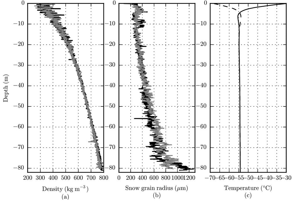
Fig. 1. (a) Snow density ( $\text{kg m}^{-3}$ ) and (b) grain size ( $\mu\text{m}$ ) profiles measured on two ice-cores at Dome C in the 2012–2013 austral summer; (c) Mean temperature profiles ( $^{\circ}\text{C}$ ) in January (solid line) and July (dashed line).
