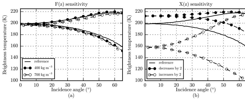
Fig. 8. Brightness temperature (K) modeled by WALOMIS with (a) the deterministic part  $F(z)$  as computed with (7) (reference, solid line), equal to  $400 \text{ kg m}^{-3}$  (black circles) and to  $700 \text{ kg m}^{-3}$  (white circles); (b) the random part  $X(z)$  as computed in Section IV-B (reference, solid line), increases by a factor two (black circles), and decreases by a factor two (white circles).
