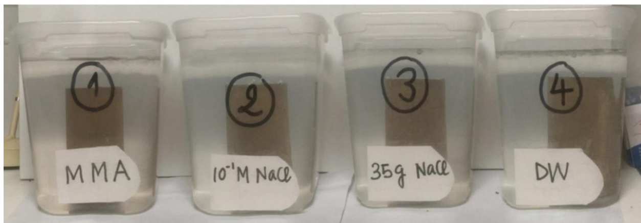
Fig. 1 Lime-treated specimens placed in four different fluids for 1 st wetting during the W-D cycles
