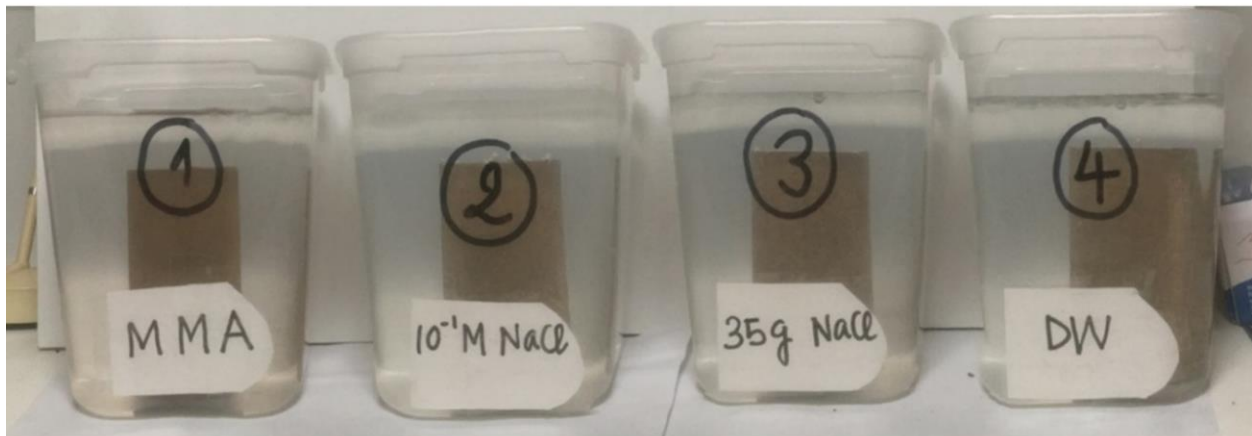
59 138 Fig. 1 Lime-treated specimens placed in four different fluids for 1 st wetting during the W-D cycles 60 61 62 63 64 65
