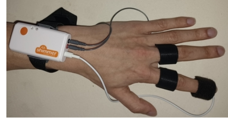
Figure 3: Shimmer3 GSR+ used to record EDA and optical pulse. Gray wires connect the EDA sensor, white wire connects the pulse sensor.
