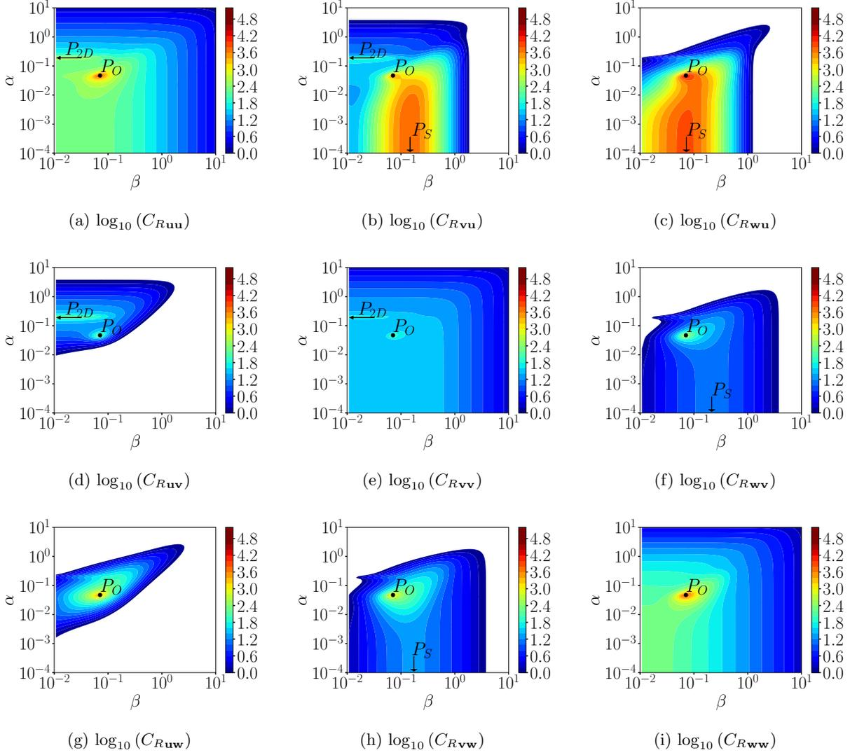
FIG. 9: Plots of the receptivity coefficients for the velocity components and  $M_\infty = 4.5$ . The subscripts indicate the input/output couple that is selected. For instance, the subscript  $\mathbf{w}\mathbf{u}$  indicates that  $\mathbf{w}$  is the input and  $\mathbf{u}$  is the output. White regions are associated with levels below 0.
