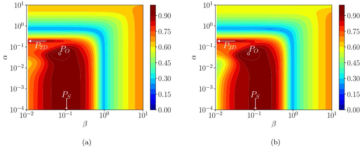
FIG. 15: The distribution of  $r_1 = \sigma_1 / \sum_j \sigma_j$  for response POD (a) and forcing POD (b) modes and  $M_\infty = 4.5$ . The subscript 1 refers to the largest eigenvalue of the correlation matrix (a) or its dual (b).
