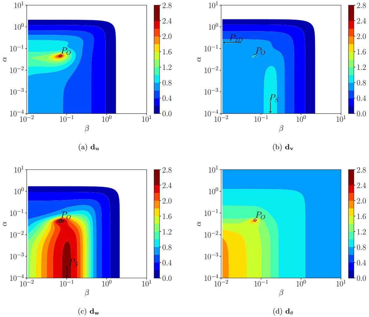
FIG. 14: Distribution of the receptivity coefficients in a logarithmic scale for various forcing components at  $y_p = 1$  and  $M_\infty = 4.5$ .
