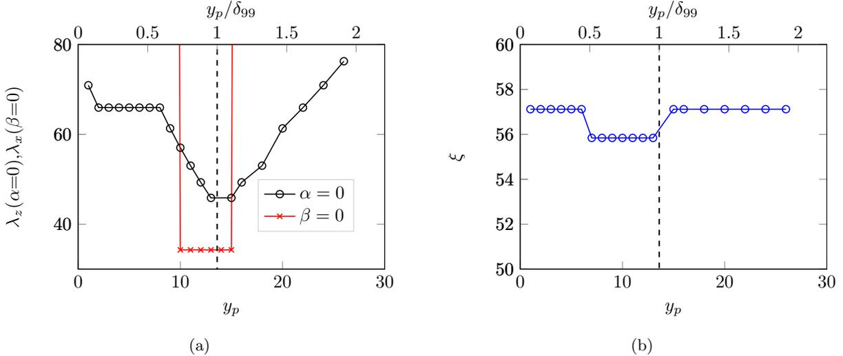
FIG. 12: Flow structure characteristics as a function of the wall-normal position of the forcing  $y_p$  for  $M_\infty = 4.5$ . (a) Characteristic wavelengths  $\lambda_z = 2\pi/\beta$ ,  $\lambda_x = 2\pi/\alpha$  for streaks and 2D flow structures ( $\alpha = 0$  and  $\beta = 0$ , respectively). The position of the  $\delta_{99}$  boundary layer thickness is shown in vertical dashed lines. (b) angle  $\xi = \arctan \beta/\alpha$  for the oblique pattern.
