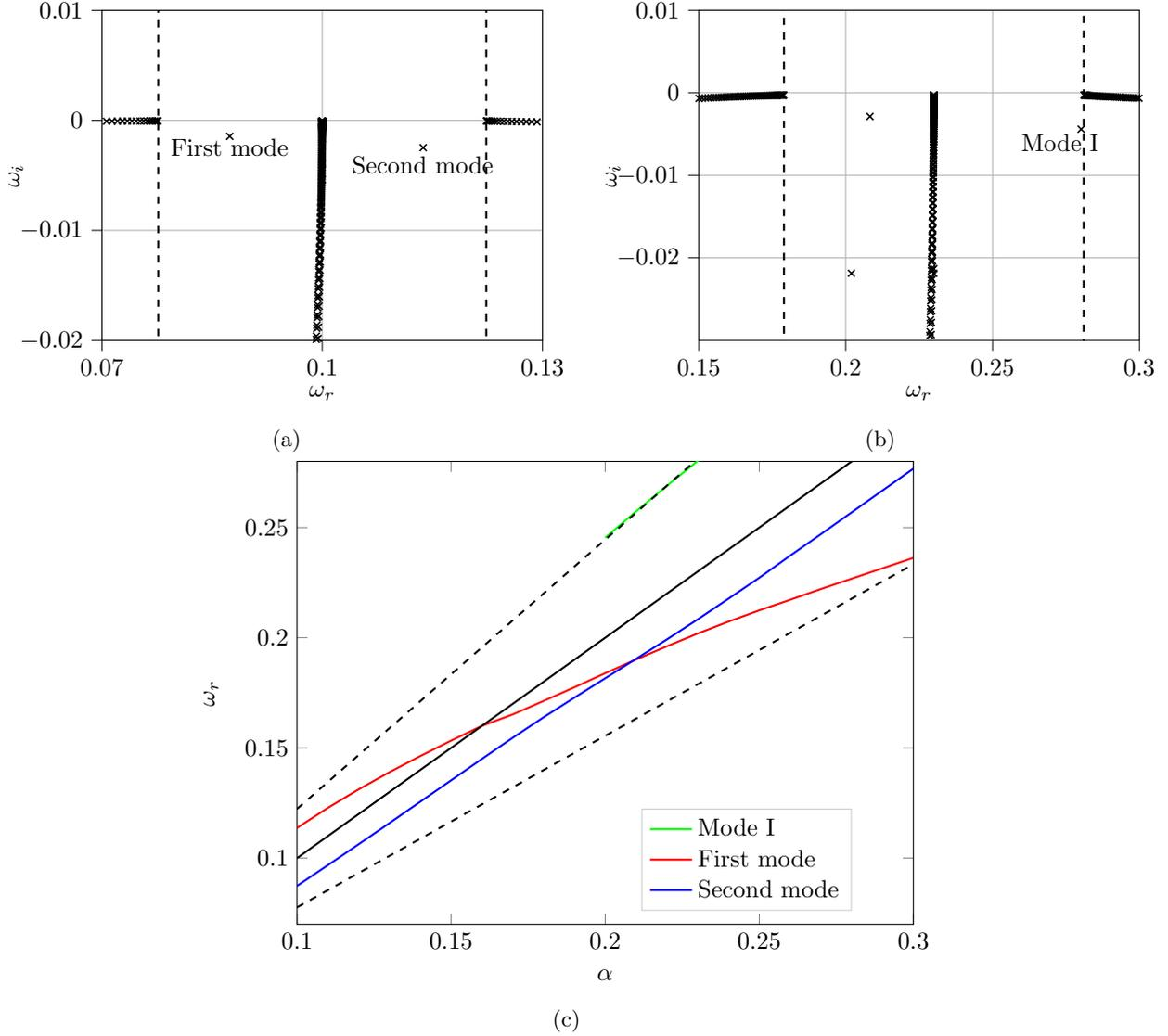
FIG. 7:  $M_\infty = 4.5$  and  $Re = 180$ . (a) and (b) spectra for  $\alpha = 0.10$  and  $\alpha = 0.23$ , respectively and  $\beta = 0$ . Panel (c) dispersion relations for the first and second modes. The discrete additional mode I (see panel (b)) is also shown. The slow and fast acoustic waves positions are represented by dashed lines. In (c), the position of the continuous branch is shown in black line.
