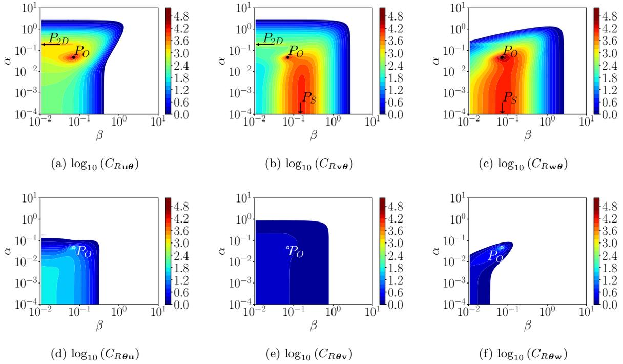
FIG. 10: Plots of the receptivity coefficients for the velocity and temperature components and  $M_\infty = 4.5$ . For details, see caption in figure 9.
