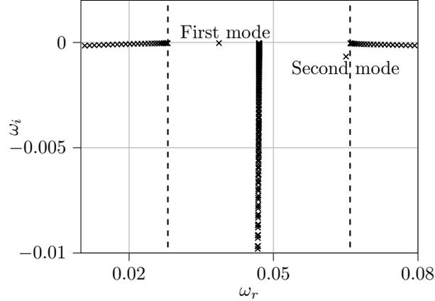
FIG. 1:  $M_\infty = 4.5$  and  $Re = 180$ . Spectrum for  $(\alpha, \beta) = (0.047, 0.071)$ , compare the cross in figure 2. Slow and fast acoustic waves positions are depicted by dashed lines.
