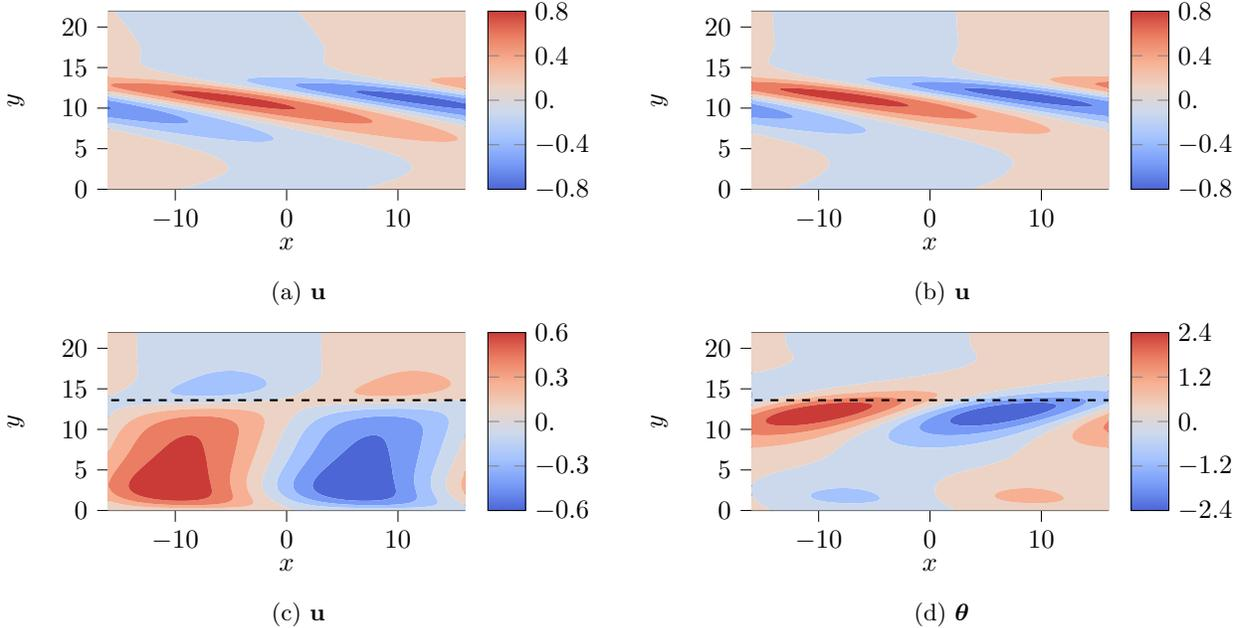
FIG. 17: Dominant forcing (a,b) and response (c,d) POD modes for  $(\alpha, \beta) = (0.19, 0)$ ,  $M_\infty = 4.5$  and the input limited to  $\mathbf{u}$ . The streamwise velocity component is shown in (a,b). The streamwise velocity and temperature components are shown in (c,d), respectively. Panels (a,c) correspond to the output measurement restricted to  $\mathbf{u}$ . Panels (b,d) correspond to the output measurement restricted to  $\boldsymbol{\theta}$ .
