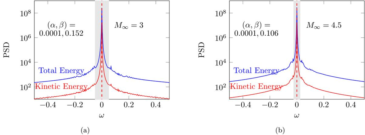
FIG. 8:  $Re = 180$ . Power spectral density plots for (a)  $(\alpha, \beta) = (0.0001, 0.152)$ ,  $M_\infty = 3$  and (b)  $(\alpha, \beta) = (0.0001, 0.106)$ ,  $M_\infty = 4.5$ . For color legends see figure 5.
