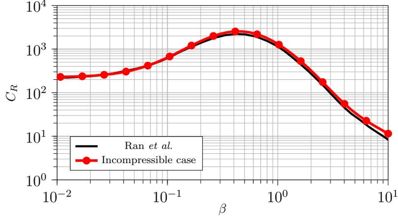
FIG. 20: The one-dimensional receptivity coefficient for the incompressible boundary layer case with  $Re = 232$ . In full black, results extracted from Ran *et al.*<sup>26</sup> are shown.
