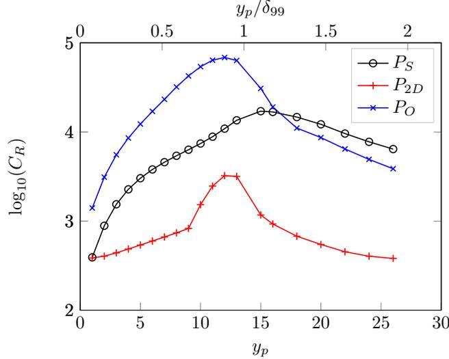
FIG. 13: Distribution of the receptivity coefficient in a logarithmic scale for  $P_{2D}$  (red),  $P_O$  (blue) and  $P_S$  (black) as a function of the wall-normal position of the input.
