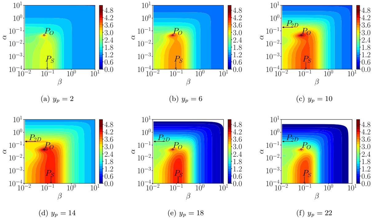
FIG. 11: Plot of the receptivity coefficients in a logarithmic scale as a function of the wall-normal position associated with the forcing for  $M_\infty = 4.5$ . The  $\delta_{99}$  boundary layer thickness is located at  $y = 13.6$ .
