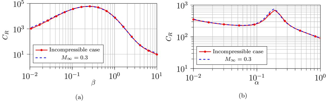
FIG. 21: Receptivity coefficient (a)  $C_R(\alpha = 0.0001, \beta)$  and (b)  $C_R(\alpha, \beta = 0.01)$  computed for the incompressible case and  $M_\infty = 0.3$  for  $Re = 232$ .
