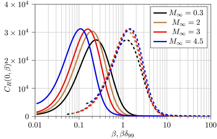
FIG. 4: Distribution of  $C_R(0, \beta)$  for the different Mach numbers and  $Re = 180$ . Full line: the reference length  $l = \sqrt{\mu_\infty x / (\rho_\infty U_\infty)}$  is used, in dashed lines data are rescaled with the  $\delta_{99}$  boundary layer thickness.
