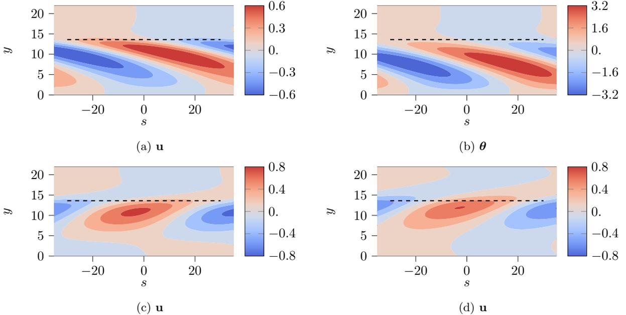
FIG. 18: Dominant forcing (a,b) and response (c,d) POD modes for  $(\alpha, \beta) = (0.04, 0.07)$ ,  $M_\infty = 4.5$  and the measurement based on  $\mathbf{u}$ . The streamwise velocity component is shown in (a,c,d). The temperature component is shown in (b). Panels (a,c) correspond to the input restricted to  $\mathbf{u}$ . Panels (b,d) correspond to the input restricted to  $\theta$ . The position in the wavevector direction is denoted by  $s$ .
