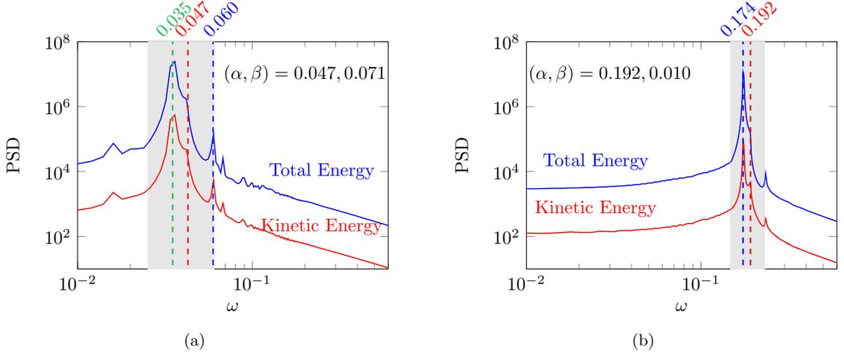
FIG. 6:  $M_\infty = 4.5$  and  $Re = 180$ . Power spectral density plots for (a)  $(\alpha, \beta) = (0.047, 0.071)$  and (b)  $(\alpha, \beta) = (0.192, 0.010)$ . The vertical lines correspond to  $\omega = 0.047, 0.060$  and  $0.035$  in (a) and  $\omega = 0.174, 0.192$  in (b). For color legends see figure 5.
