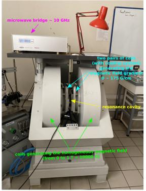
(a) X-band EPR 2D imaging system
