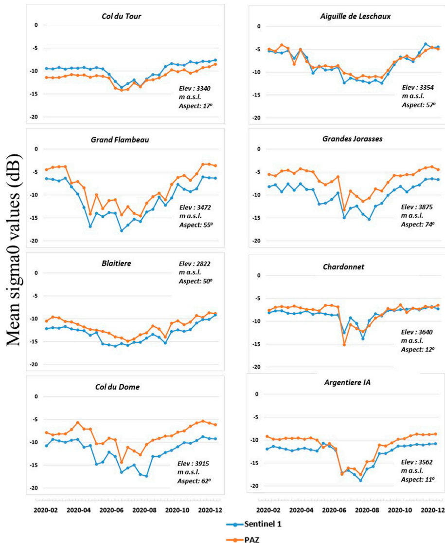
FIGURE 12 | Comparison of the temporal backscattering profiles for 8 IAs in X-band PAZ and C-band interpolated Sentinel-1 images.
