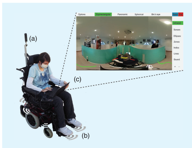
Figure 6. The basic system components of SpheriCol. The (a) twin-fisheye camera, (b) wheelchair equipped with a ring of ToF sensors, and (c) user interface displaying a panoramic image of the surrounding environment, with colored distance markers overlaid.
