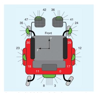
**Figure 3.** The wheeled platform developed at INSA Rennes (top view). The ID and location of the 48 ToF sensors mounted on the wheelchair are shown. The seven sensor modules are depicted in green.
