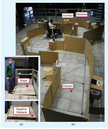
**Figure 11.** UCL's PAMELA facility. (a) The modular platform enables setting up slopes and negative obstacles. (c) The circuit, with a volunteer testing the model-based shared control algorithm proposed in [26].
