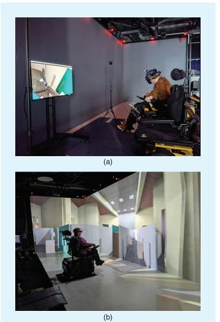
Figure 4. A wheelchair simulator tested by a volunteer in immersive conditions. In (a), the user wears a head-mounted display, and in (b), the user wears 3D glasses in *Immersia*, a virtual-reality research platform at IRISA/Inria Rennes.
