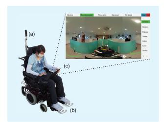
**Figure 6.** The basic system components of SpheriCol. The (a) twinfisheye camera, (b) wheelchair equipped with a ring of ToF sensors, and (c) user interface displaying a panoramic image of the surrounding environment, with colored distance markers overlaid.
