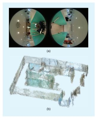
**Figure 5.** (a) A dual-fisheye image captured by a Ricoh Theta S camera. (b) An image-based 3D reconstruction of the obstacle course at Pôle Saint-Hélier (a physical medicine and rehabilitation center in Rennes), obtained with Metashape. The ceiling has been removed to provide visibility of the room interior.
