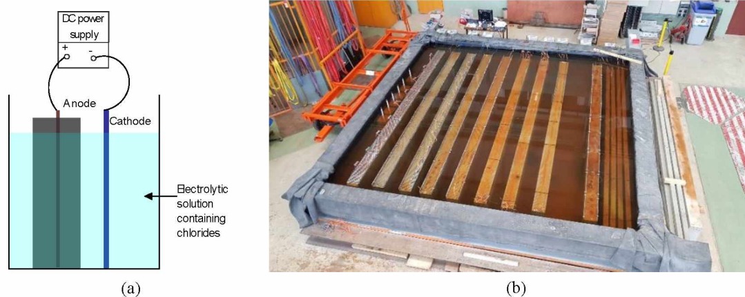
Figure 2: Accelerated corrosion technique: (a) Simplified setup, (b) Corrosion of the specimens.
