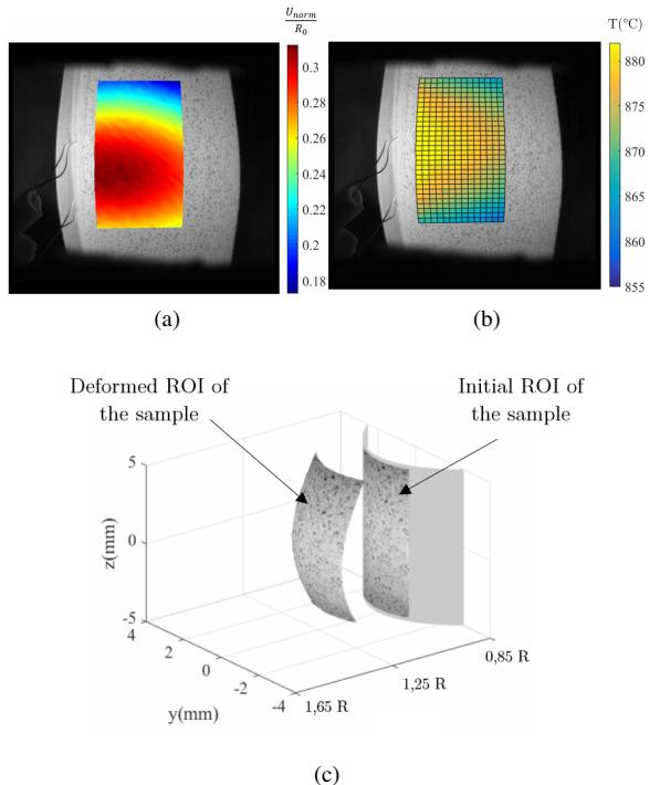
Figure 10: Example of results obtained during a test performed at  $880 \text{ } ^\circ\text{C}$  and 11 bar: (a) displacement field computed by stereo-correlation and normed by the initial radius of the sample  $R_0$ ; (b) thermal field obtained by NIR thermography; (c) 3D reconstruction of the ROI.
