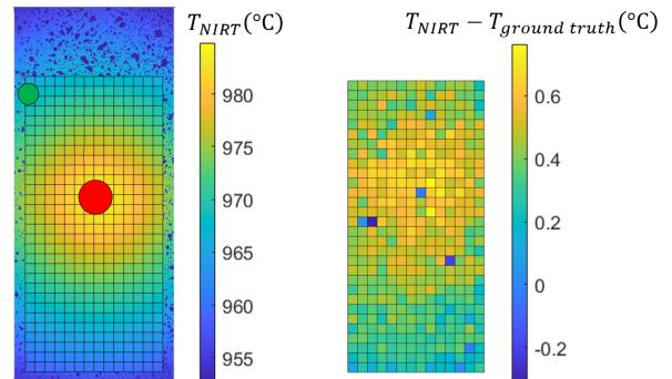
Temperature field obtained by thermography on the DIC mesh
