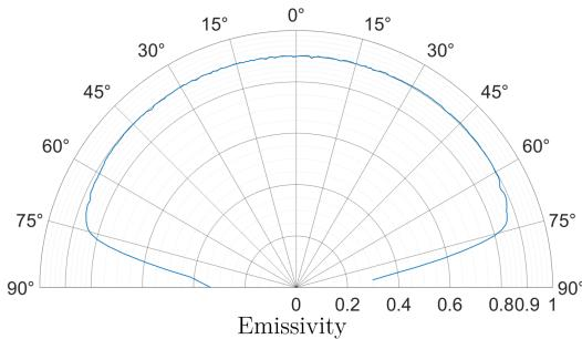
Figure 13: Evolution of the emissivity with the observation angle. The emissivity at  $0^\circ$  is here arbitrary set equal to 0.9. These results were obtained using the black paint on a sample heated to  $1000\text{ }^\circ\text{C}$ .
