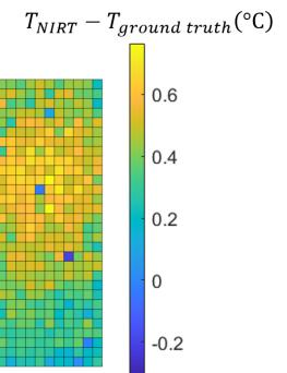
Difference between the temperature obtained by thermography and the true temperature
