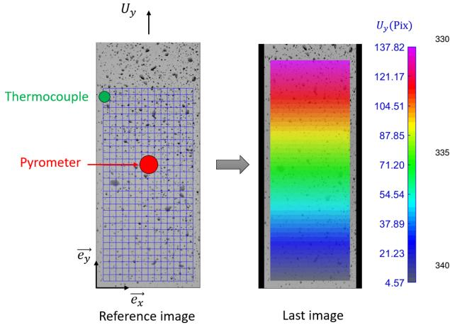
Figure 2: Example of an image obtained from a real experiment performed at 950 °C. The virtual pyrometer and thermocouple locations are shown in red and green, respectively. The deformed image generated for the last step of the virtual test case is also presented with the y-displacement field.
