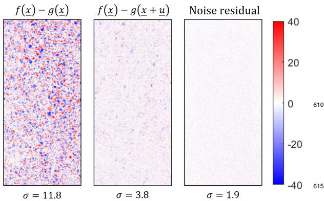
Figure 11: Residual maps obtained during the tests at the first and last iteration of the DIC algorithm (two left maps). The right map shows the approximated residual map solely caused by noise. The error is expressed in gray level.
