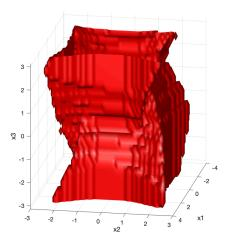
Figure 2. Controlled invariant  $X_I$  computed using symbolic control techniques.
