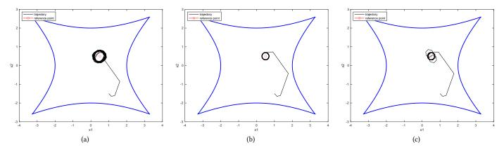
Figure 3. For reference position  $x^r = (0.5, 0.5)$ , closed-loop trajectories with OSC (a), MPC (b), SgMPC (c).
