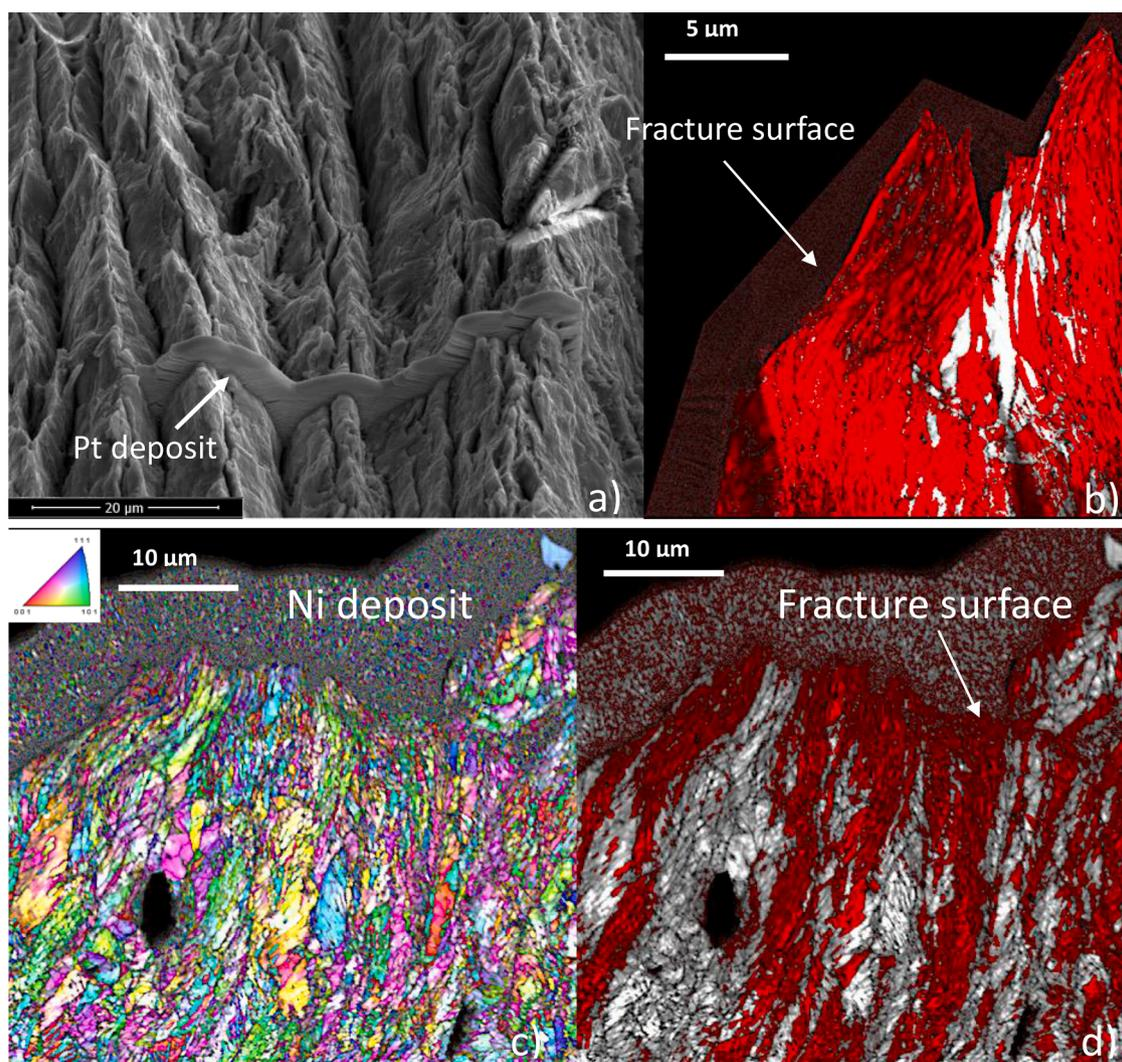
**Fig. 1.** 316L-Hg (a) Tilted SEM view of the FIB sampling area with the protective platinum deposit before FIB sectioning (b) t-EBSD phase map of the FIB lamella with Image Quality (IQ) gray coding ( $\alpha'$  iron in red) (c) Inverse pole figure (IPF) + IQ map of the coarse-grained cross section (d) Corresponding coarse-grained phase map with IQ gray coding relative to (c) ( $\alpha'$  iron in red). All images are taken from slow strain rate CCT samples at room temperature.
