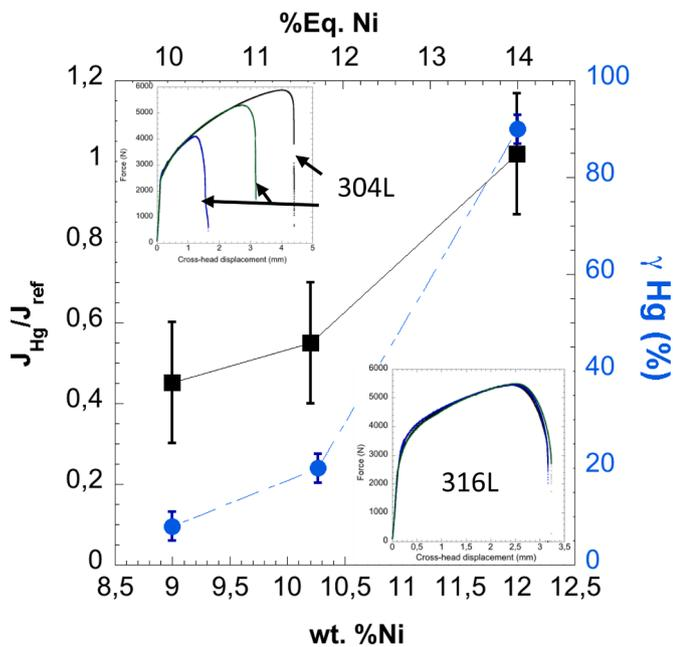
**Fig. 3.** Left) Energy to fracture normalized to the reference test (in black). Right) Quantification of the  $\gamma$  phase by X-Ray fractography (in blue). Upper left insert) Force versus Cross-head displacement curves for 304 L austenitic steel (Blue and green in contact with mercury). Lower right insert) Force versus Cross-head displacement curves for 316L(N) austenitic steel.
