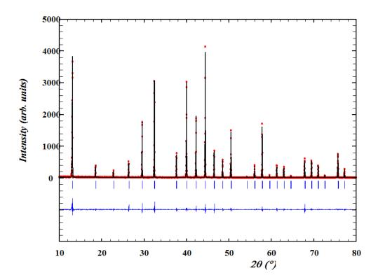
**Figure 1.** Rietveld refinement of the powder X-ray diffraction diagram for NaMo<sub>6</sub>Se<sub>8</sub>. The experimental data are shown in red and the calculated profile is represented in solid black line. The difference profile between the theoretical and experimental patterns is represented in blue. The vertical blue ticks indicate the Bragg reflection positions.
