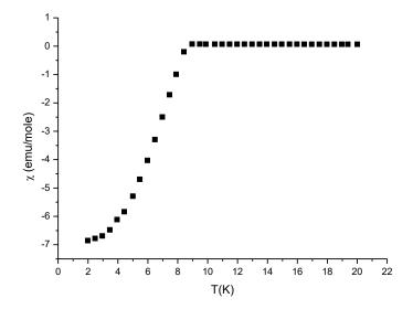
Figure 7. Temperature dependence of the magnetic susceptibility of  $NaMo_6Se_8$  below 20 K.
