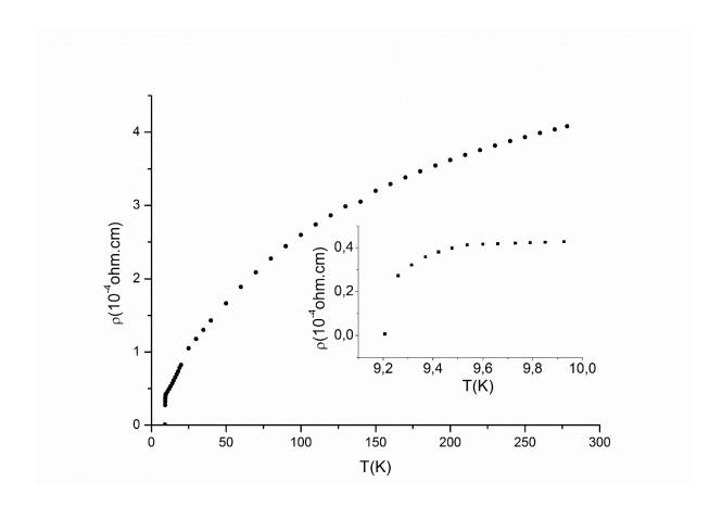
**Figure 6.** Temperature dependence of the electrical resistivity  $\nearrow$  of a NaMo<sub>6</sub>Se<sub>8</sub> single-crystal.
