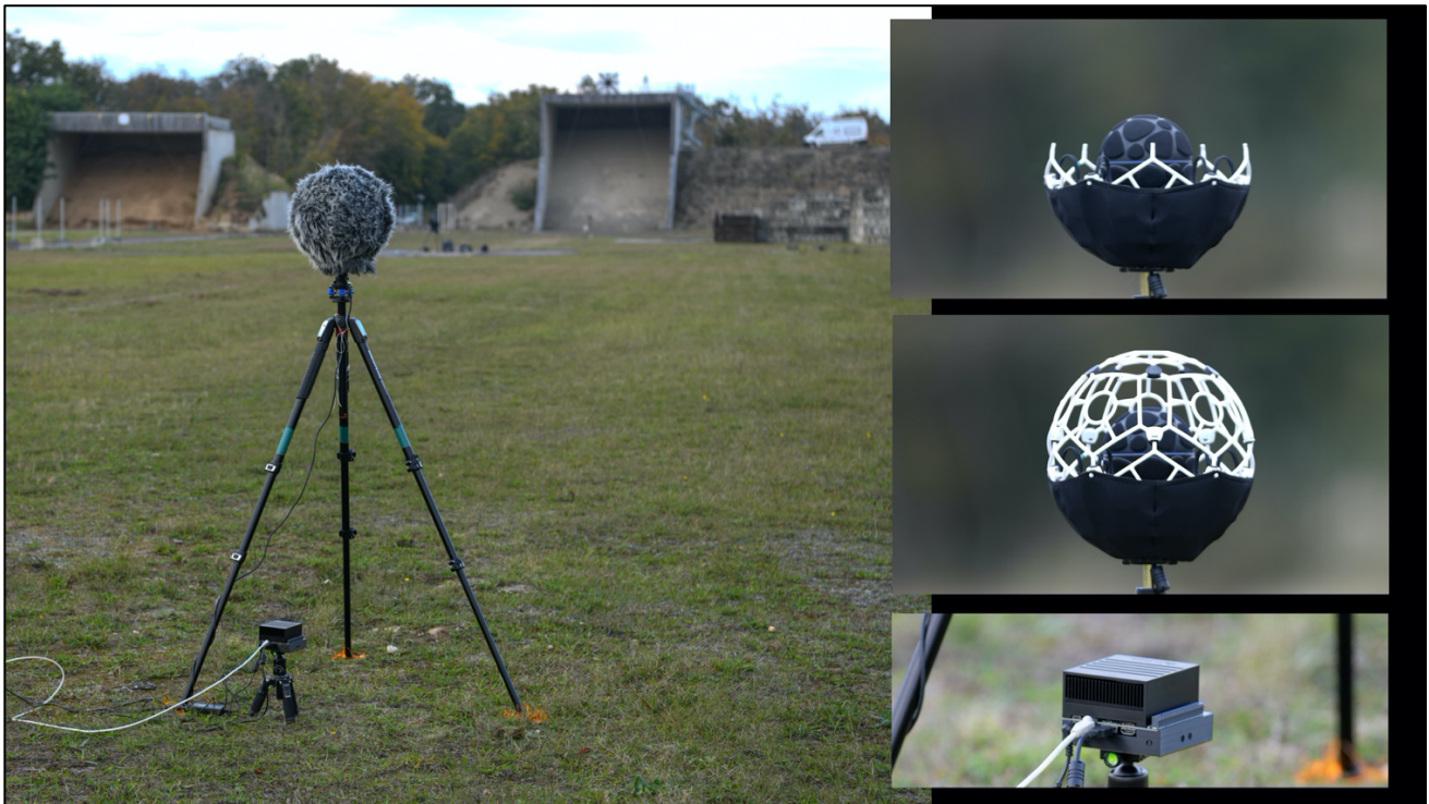
Figure 2: AI-enhanced MEMS microphone array used in the project, with a compact, low-power AI processor (bottom right).
