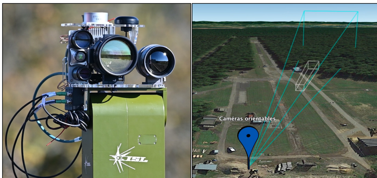
Figure 3: Left: The optronic system composed of various cameras (visible, thermal, and active imaging) mounted on a servo-turret. Right: On-site field of view of the various cameras used in the optronic system. Cyan: visible field of view. White: active imaging field of view. The active imaging range is selectable and controlled by the fusion unit which processes the inferred UAV positions transmitted in real time by the acoustic monitoring nodes.
