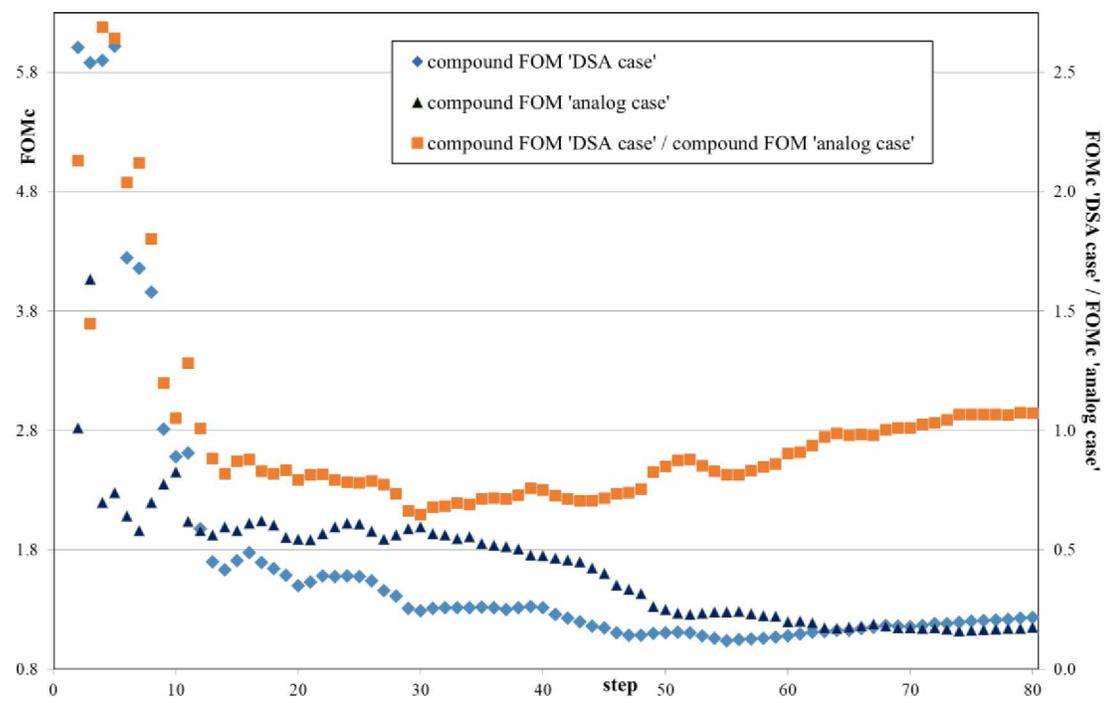
Figure 20. PWR Gen III; fast neutron flux on PV at 0° below supporting platforms (increasing no. fission neutrons passing from fictitious to real-world source cells):  $FOM_c$ 's of the 17 in-core global responses for the two approaches, “DSA” and “analog”, and their ratio
