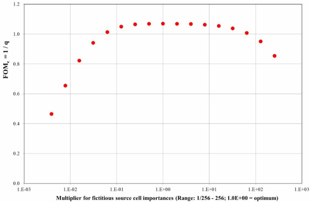
Figure 8. PWR Gen III; ex-core mapping of the neutron flux (increasing no. fission neutrons passing from fictitious to real-world source cells): inverse of the quality (2<sup>nd</sup> moment × time) against multiplier of the fictitious source cell importances
