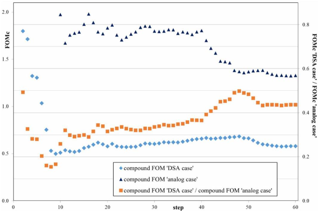
Figure 12. PWR Gen III; ex-core mapping of the neutron flux (increasing no. fission neutrons passing from fictitious to real-world source cells):  $FOM_c$ 's of the 15 in-core global responses for the two approaches, “DSA” and “analog”, and their ratio
