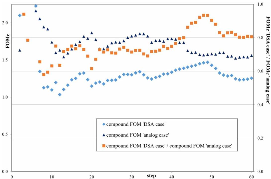
Figure 9. PWR Gen III; ex-core mapping of the neutron flux (increasing no. fission neutrons passing from fictitious to real-world source cells): ex-core local responses group A,  $FOM_c$ 's of the two approaches, "DSA" and "analog", and their ratio
