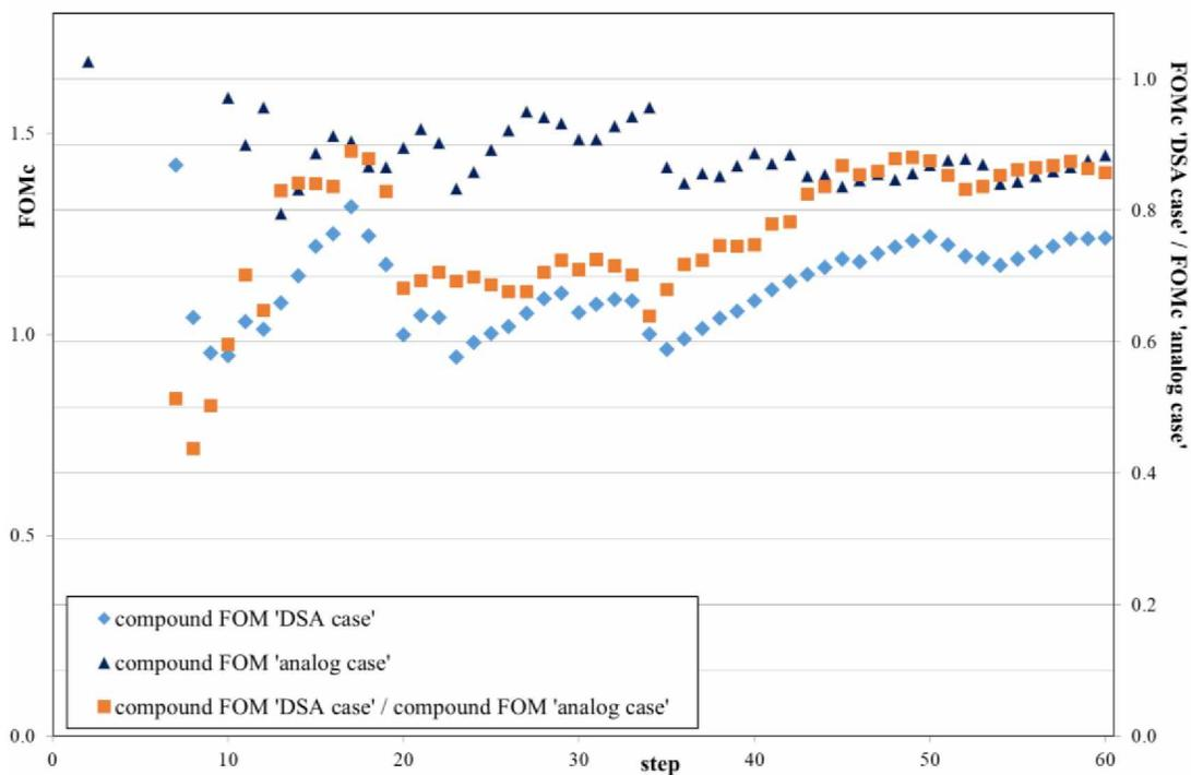
Figure 10. PWR Gen III; ex-core mapping of the neutron flux (increasing no. fission neutrons passing from fictitious to real-world source cells): ex-core local responses group B,  $FOM_c$ 's of the two approaches, "DSA" and "analog", and their ratio
