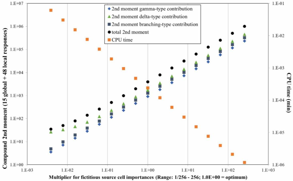
Figure 7. PWR Gen III; ex-core mapping of the neutron flux (increasing no. fission neutrons passing from fictitious to real-world source cells): 2<sup>nd</sup> moment and time against multiplier of the fictitious source cell importances
