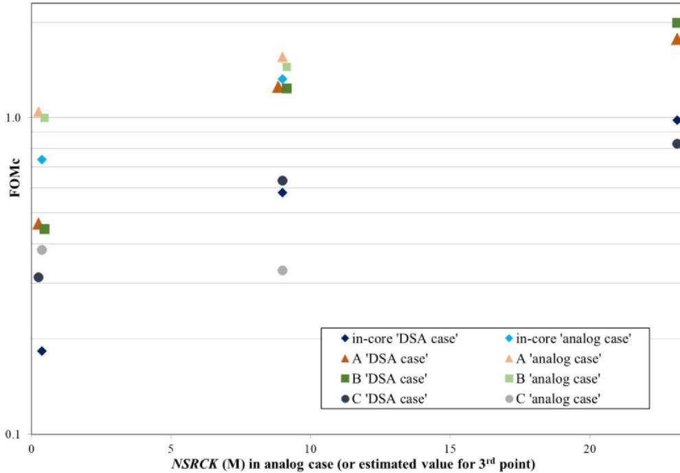
Figure 13. PWR Gen III; ex-core mapping of the neutron flux: final  $FOM_c$ 's of the two approaches, "DSA" and "analog", for the 15 in-core global responses and the three groups of local ex-core responses for the results in Figs. 3-6 and 9-12 and in this section with a  $NSRCK$  value of  $9 \times 10^6$  in the DSA approach
