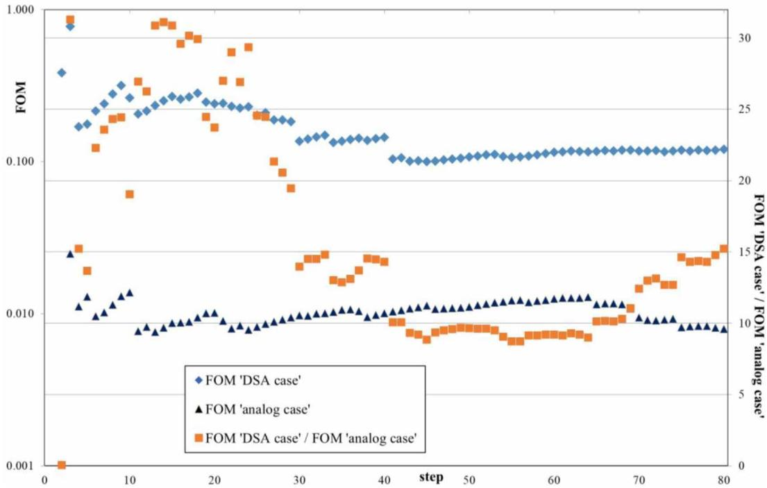
Figure 19. PWR Gen III; fast neutron flux on PV at 0° below supporting platforms (increasing no. fission neutrons passing from fictitious to real-world source cells):  $FOM$ 's of the ex-core response for the two approaches, “DSA” and “analog”, and their ratio
