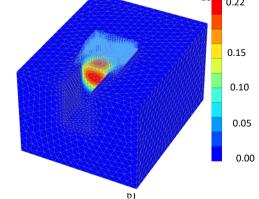
Figure 20. a) Photo of the scoop pressing above the pit; b) Finite element model with incremental displacement contours for the flat push (Vrettos 2022, pers. comm.).
