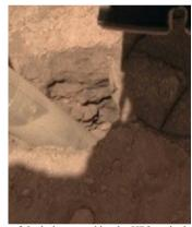
Figure 11. Image of the hole created by the HP3 mole during hammering (inclined  $\sim$ 15°), with the scoop appearing on top right (image credit JPL/NASA).
