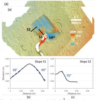
Figure 21. (a) Digital elevation model of the HP<sup>3</sup> pit based on the stereo pair taken on Sol 673 erter scraping; (b) Elevation profile S1 of the scrapsedian(d)Elevation pairitate prone Sola673 withen scraping al. 20(b)Splowation2p2001 E S1 of the scraped pile (c) Eleva-
