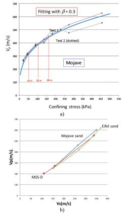
Figure 13. Bender elements measurements of velocity waves: a) changes in  $V_p$  with confining stress; b) linear relation between  $V_p$  and  $V_s$  for the three simulants investigated. A common value v = 0.22 is obtained for the three simulants tested (Delage et al. 2017).
