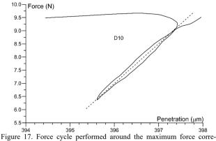
Figure 17. Force cycle performed around the maximum force corresponding to the force supported by a SEIS foot. The cycle is fairly reversible illustrating satisfactory elastic response under the imposed displacement (around 2  $\mu$ m). Its slope provides the elastic spring constant  $k_v$  used in the analysis of the dynamic interaction between SEIS and the ground (Delage et al. 2022)
