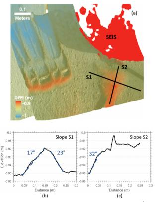
Figure 22. (a) Digital Elevation Model of the surface between HP<sup>3</sup> and SEIS based on the stereo pair taken on Sol 877 after scraping, scooping and dumping; (b) Elevation profile S1 of the dumped pile; (c) Elevation profile S2 of the dumped pile (Marteau et al. 2022).
