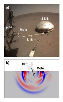
Figure 18. a) Image taken on June 28, 2019 (sol 209) showing how the HP<sup>3</sup> support structure was lifted and revealing the partially buried mole (see Figure 11), located around 1.18 m away from InSight's seismometer SEIS (image credit JPL/NASA); b) Conceptual illustration of the HP<sup>3</sup> mole generating seismic waves (blue and red colors correspond to negative and positive amplitudes) propagating through the shallow subsurface at the InSight landing site (Brinkman et al. 2022).
