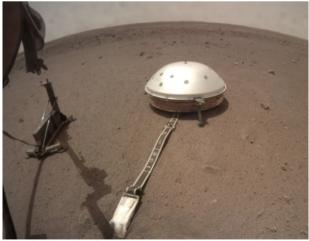
Figure 3. Photo taken from the Instrument Context Camera (ICC) showing the location of SEIS and of the HP<sup>3</sup> support structure, 1.18 meter apart from each other (image credit JPL/NASA).
