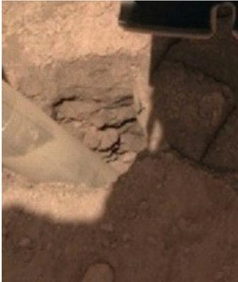
Figure 11. Image of the hole created by the HP3 mole during hammering (inclined ~15°), with the scoop appearing on top right (image credit JPL/NASA).
