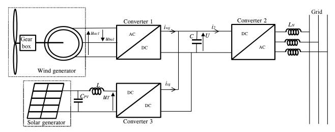
Fig 1. Hybrid wind-photovoltaic generating system.
