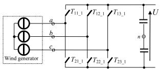
Fig. 2: Electrical diagram of the converter 1
