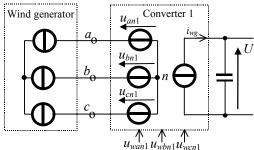
Fig. 4: Equivalent electrical diagram of the converter 1
