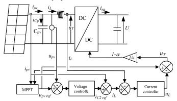
Fig. 9. Control of the photovoltaic system.
