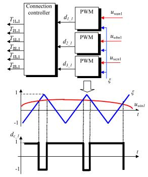
Fig. 3. Classical PWM method: comparison between a reference wave  $u_{win1}$  and a modulation wave  $\xi$ .
