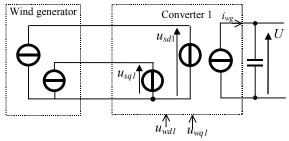
Fig. 5: Equivalent electrical diagram of the converter 1 in the d,q frame
