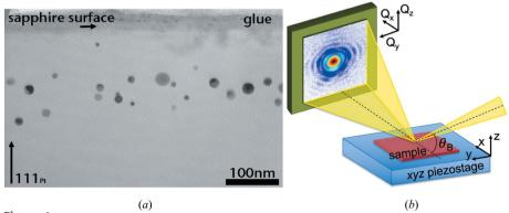
Figure 1 (a) Transmission electron microscopy image of a  $c(0001)_{\alpha}$  substrate implanted with  $1 \times 10^{16} \, \text{Pt}^+ \, \text{cm}^{-2}$  at room temperature and after annealing at 1873 K for 100 h. The  $[0001]_{\alpha}$  crystallographic direction points vertically. (b) A scheme of the experimental setup.
