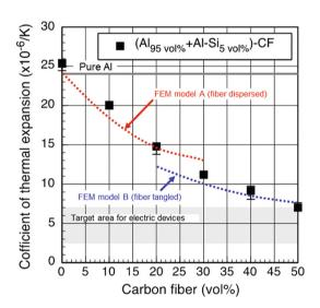
Fig. 6 CTEs of (Al<sub>95 vol%</sub> + Al-Si<sub>5 vol%</sub>)– and Al–CF composites in the in-plane direction of the carbon fibers
