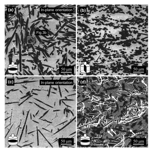
Fig. 2 SEM micrographs of  $(Al_{95\ vol\%} + Al-Si_{5\ vol\%})$ – $CF_{50\ vol\%}$  composite in the in-plane **a** and transverse directions **b** of the carbon fiber, **c**  $(Al_{95\ vol\%} + Al-Si_{5\ vol\%})$ – $CF_{20\ vol\%}$  composite in the in-plane direction of the carbon fiber, **d**  $Al-CF_{50\ vol\%}$  composite in the in-plane direction of carbon fiber
