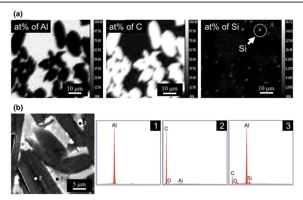
Fig. 3 Results of microanalysis: a EPMA mapping, b EDX spot scan in (Al<sub>95 vol%</sub> + Al-Si<sub>5 vol%</sub>)-CF<sub>50 vol%</sub> composite
