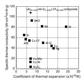
Fig. 9 Specific thermal conductivities versus CTE of several materials selected as heat sink materials
