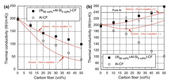
Fig. 5 Thermal conductivities of (Al<sub>95 vol%</sub> + Al–Si<sub>5 vol%</sub>)– and Al–CF composites in the transverse direction a and in-plane direction b of the carbon fibers
