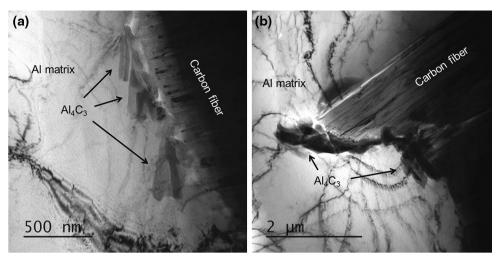
Fig. 7 TEM micrographs of (Al $_{95\ vol\%}$  + Al $_{95\ vol\%}$ )-CF $_{50\ vol\%}$  composite: a Al/CF interface, b tip of the carbon fiber
