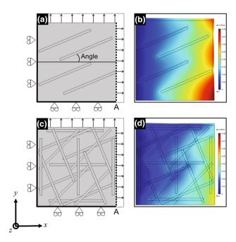
**Fig. 8** FEM calculation images: **a** calculation criteria, **b** the displacement after calculation of (Al<sub>95 vol%</sub> + Al–Si<sub>5 vol%</sub>)–CF<sub>10 vol%</sub> composite without the tangles of carbon fibers, **c** calculation criteria, **d** displacement after calculation of (Al<sub>95 vol%</sub> + Al–Si<sub>5 vol%</sub>)–CF<sub>50 vol%</sub> composite with tangles of carbon fibers
