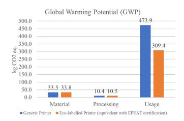
Fig. 5. Comparison of the carbon footprint of the two printers
