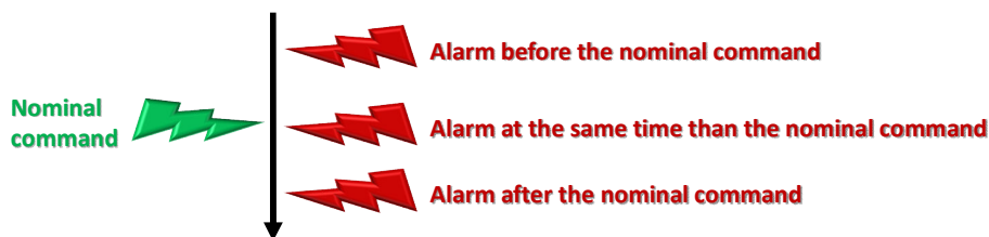
Figure 7 : Automatic Test Generation: Robustness tests
