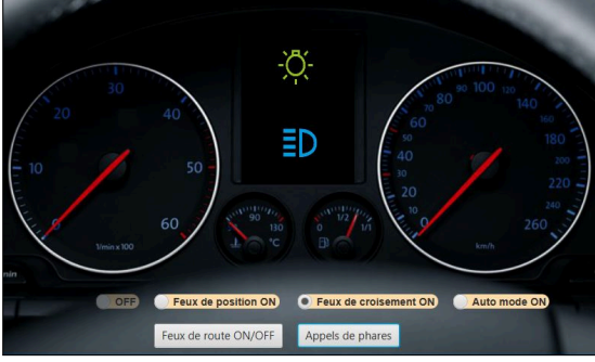
Fig. 4. Example of Graphical User Interface associated to a Java simulation of the AFLS.
