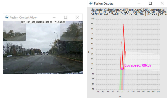
Fig. 11: Fusion Control View and Fusion Display windows at step 4217.
