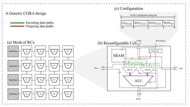
Illustration of a simple CGRA taken from [48], showing the mesh topology (a), the internal architecture of the Reconfigurable Cell, RC (b), and an example of the configuration register (c).
