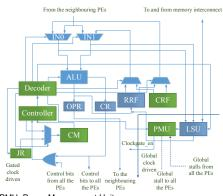
PMU: Power Management Unit RRF: Regular Register file CRF: Constant Register File
