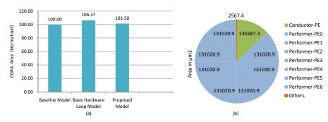
Fig. 9 (a) Synthesized area of IPA PE array in different implementations; (b) Area breakdown of IPA (4X2) in the proposed model
