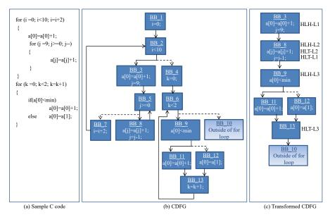
$\textbf{Fig. 7} \hspace{0.1in} \textbf{(a) Sample program; (b) Corresponding CDFG; (c) Transformed CDFG}$
