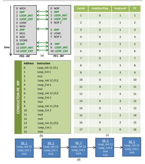
**Fig. 5** (a) Snapshot of PE IRFs holding temporally synchronized instructions; (b) Conductor-PE IRF with a sample pseudo-code; (c) Log of register updates according to the pseudo-code in (b)
