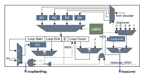
Fig. 4 Hardware Loop Block in the Conductor-PE
