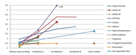
Fig. 10 Gain in latency achieved against the baseline model by applying loop unrolled kernels on the proposed model
