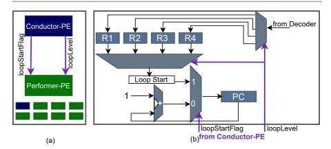
$\textbf{Fig. 3} \hspace{0.1in} \textbf{(a)} \hspace{0.1in} \textbf{Conductor-Performer Model; (b)} \hspace{0.1in} \textbf{Hardware Loop Block in the Performer-PEs}$
