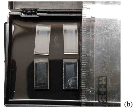
Figure 9. (a) Signal beam energy and M^2 calculated at the output of the OPA line as a function of pump energy in the first OPA stage. The configuration is composed of two stages with two PPKTP crystals in each stage and idler filtering. The total pump energy distributed in the OPA line (stage 1+2) is 200 mJ. (b). Picture of 4 PPKTP crystals.
