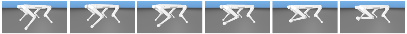
Fig. 3: Randomized-DDP leverages the smooth dynamics to precisely schedule movements requiring to break contacts.
