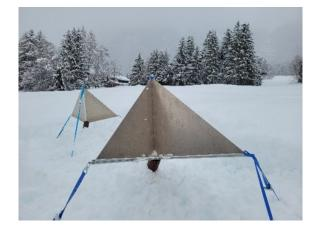
Figure 2. Corner reflectors installed in Chamonix valley, January-June 2021. Picture taken on 15/01/2021 (the first date of CR installation).
