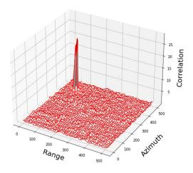
Figure 10. Correlation peak measured between 2 PAZ 64x64 pixel patches oversampled by a factor of 8 by zero padding.
