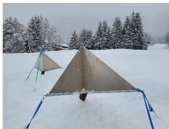
Figure 2. Corner reflectors installed in Chamonix valley, January-June 2021. Picture taken on 15/01/2021 (the first date of CR installation).
