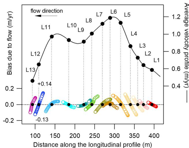
**FIGURE 3** Average velocity profiles plotted according to the distance along the longitudinal profile (cubic spline black curve) and the associated bias affecting velocity changes due to block displacements. Open circles plot the annual velocity changes attributable to the travel of blocks during the recorded period. Biases are indicated for block L12 (see text) [Colour figure can be viewed at [wileyonlinelibrary.com](http://wileyonlinelibrary.com)]
