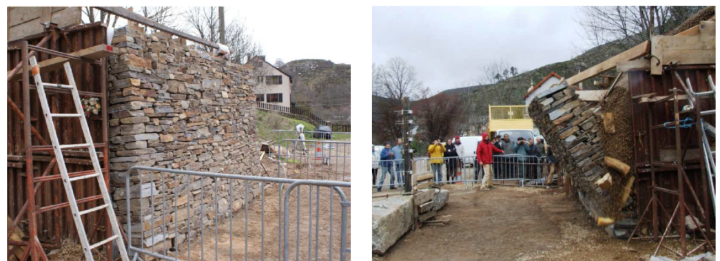
Figure 8. Picture of the “C3s” DSRWs tested by A.S. Colas: initial and collapse configurations are shown [43].
