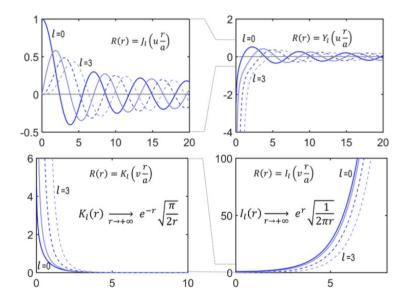
**Figure A5.** Bessel functions of the first and second kinds  $J_l$  and  $Y_l$  (left), and modified Bessel functions of the second and first kinds  $K_l$  and  $I_l$  (right), for l = 0, 1, 2, 3, from [108].
