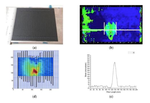
**Figure 16.** (a) Composite laminate with optical fiber following parallel paths; (b) Ultrasonic C-scan of the impacted laminate; (c) Strains measured by optical backscatter reflectometry along the white line (position of the optic fiber) of the upper figure; (d) Strain plotting at the delaminated area, obtained by parallel optical fibers, from [84].
