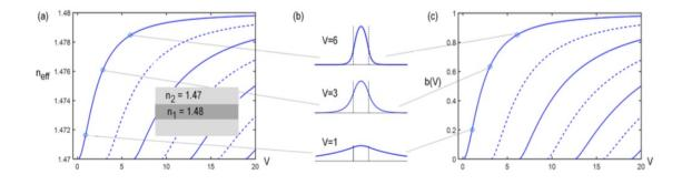
Figure A4. Evolution of the effective index  $n_{eff}$  (a), fundamental mode profiles (b), and reduced propagation constant b as a function of the reduced frequency V, from [108].
