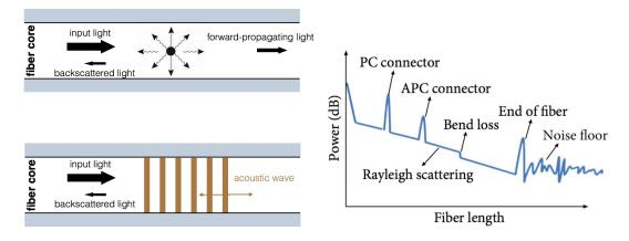
Figure 3. Schematic of Rayleigh (top left) and Brillouin (bottom left) scatterings, and typical curve of back-detected power as a function of time/distance (right).
