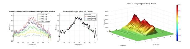
Figure 13. Strains measured by the DOFS on the embedded segment (left), and interpolated measured strain at the embedded segment (right), from [24].
