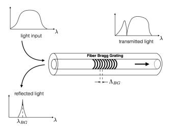
Figure 5. Illustration of the FBG principle.
