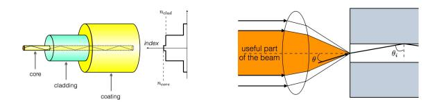
Figure 1. Geometry of a step-index optic fiber (left), with total internal reflection in the core and numerical aperture of the obtained waveguide (right).
