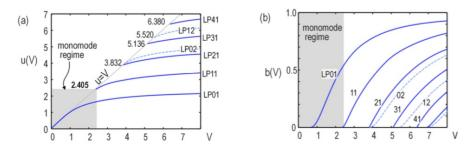
**Figure A6.** First  $LP_{lm}$  modes with functions u(V) (a) and b(V) (b), from [108].
