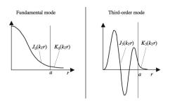
Figure A7. Radial repartition for two modes of a step index fiber.
