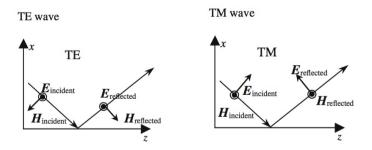
Figure A2. Respective positions of electric and magnetic fields for TE and TM waves.
