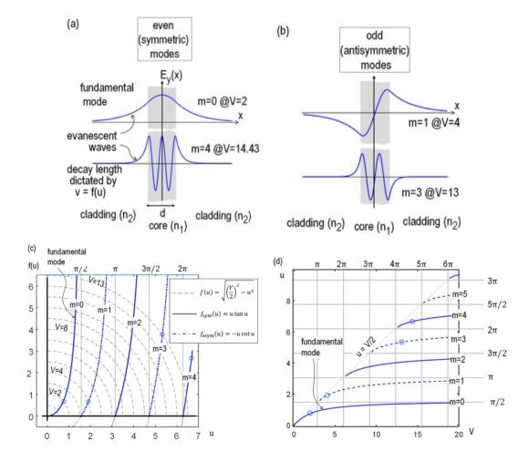
Figure A3. Illustration of modes for a symmetric step-index planar waveguide, with selected even (a) or odd (b) modes for indicated values of m and V, graphical determination of u(V) (c), and solutions in the form u(V) (d), from [108].
