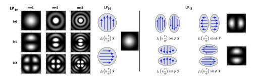
**Figure A8.** Intensity distributions of the  $LP_{lm}$  modes (left), and schematic field pattern of  $LP_{01}$  and  $LP_{11}$  modes (right), from [108].
