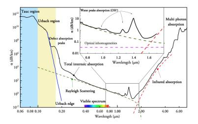
Figure 2. Attenuation with respect to wavelength in a typical silica optic fiber (from [35]).
