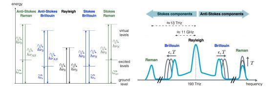
**Figure 4.** Schematic representation of energy exchanges for Rayleigh, Raman and Brillouin scatterings (left), and of the associated spectral components (right).
