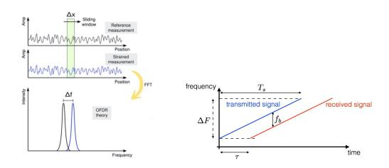
**Figure 9.** Working principle of Rayleigh backscattering optical fiber sensors based on OFDR.
