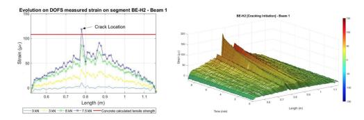
Figure 12. Detection of cracking at the surface of the concrete beam (left), and evolution of strains verified for segment BE-H2 (right), from [24].
