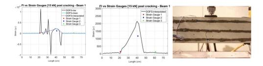
Figure 15. Comparison of the DOFS values (before and after interpolation) with strain gauges, and picture of the beam specimen with highlighted crack, from [24].
