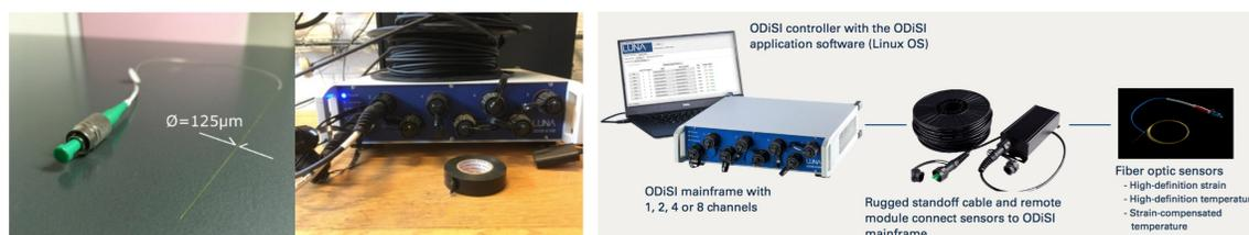
**Figure 10.** DOFS fiber and ODiSI system from LUNA Innovations.
